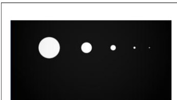
a) Example of a gauge with 5 holes of different diameters from 50-10000 \mu\text{m} in a gold layer.
